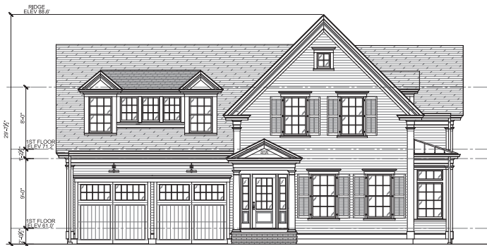
1 - NORTH EXTERIOR ELEVATION SCALE: 3/16" = 1'-0"
