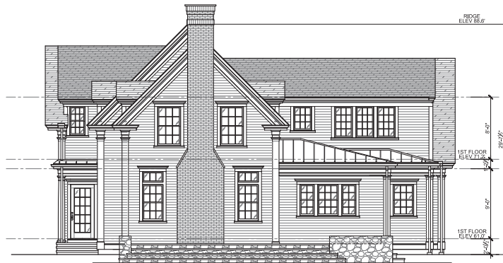
3 - SOUTH EXTERIOR ELEVATION SCALE: 3/16" = 1'-0"
