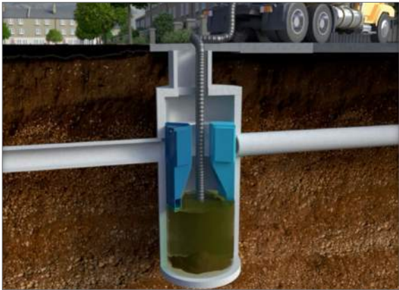
Fig.2 Maintenance is performed with a vector truck.
